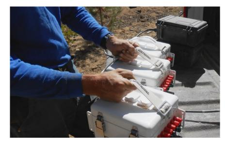
Designed for high-performance and reduced deployment costs in the collection of MT data, the new ZEN High-Res Receiver™ collects the highest resolution data currently possible and weighs less than 6 pounds (2.6kg).
