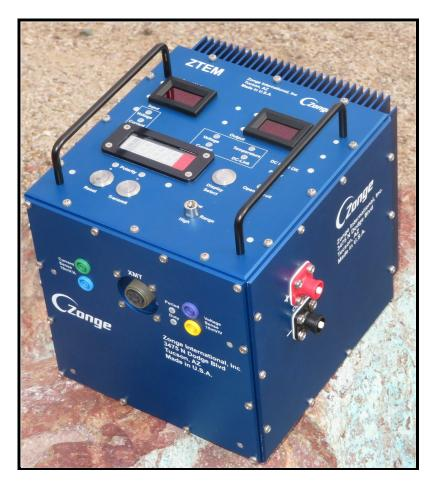
The ZTEM30 is a transmitter capable of producing time-domain or frequency-domain waveforms into either resistive or inductive loads. As a TEM transmitter, the ZTEM30 can deliver up to 30A into a 100m loop with a turnoff time of less than 200  $\mu$ s. Because the ZTEM-30 also performs well while transmitting into resistive loads, some customers can use it as a low-power resistivity transmitter. FEATURES
